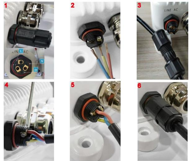
(1) The AC input port is screw terminal connector, on the AC input port there is an indicator showing pin definition. The 3 pins are labelled: Ground, N (neutral) and L (line).
